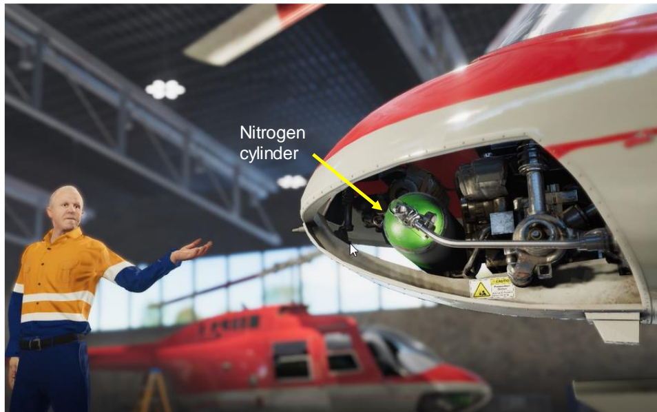
Fig. 1: Bell 412 helicopter, registration VH-BBB, showing the position of the cylinder in the nose section of the aircraft.
